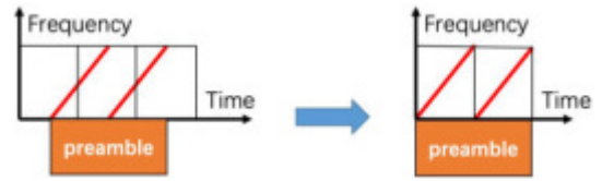
Fig. 7. Align chirps of the preamble with time window.
