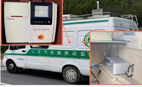
Fig. 9. Deployment of Sensing Front-ends and mass spectrometer on a mobile vehicle.
