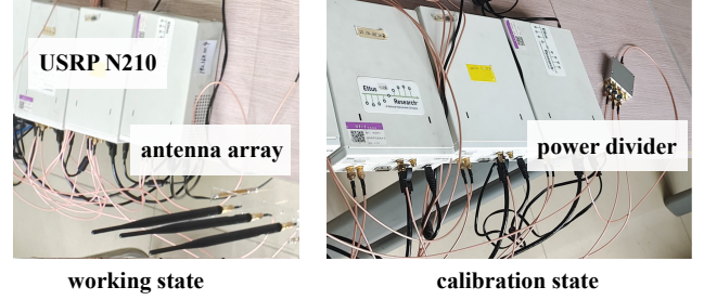
Figure 3. Traditional calibration methods may involve changing the connection state of the hardware.
